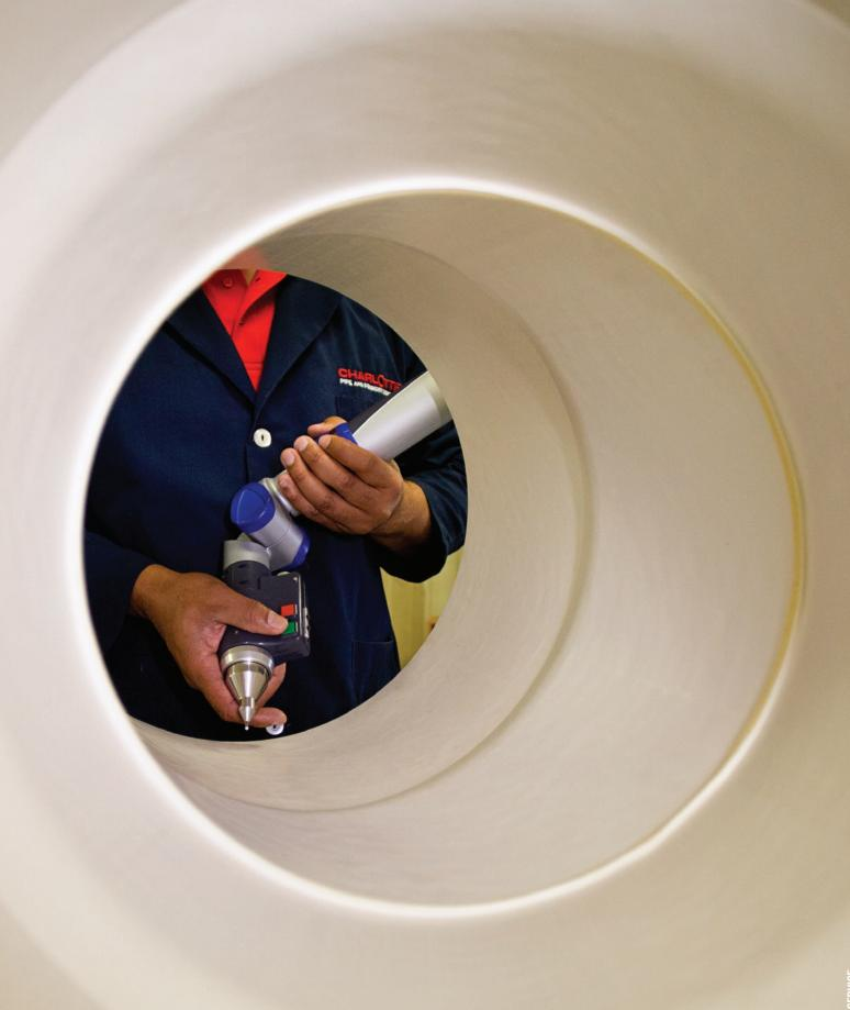
At Charlotte Pipe, our Quality Control is second to none. All our pipe and fittings are checked for dimensional accuracy and chemical composition. We also perform regular hydrostatic burst, crush and impact-strength tests to be sure we meet our goal of producing the highest-quality products possible.
